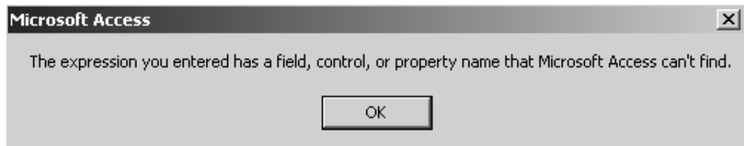
Fig 8.4.8 error message if a field is missing from the Crosstab query.
