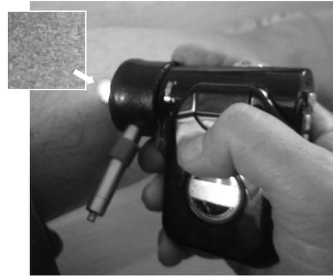
Fig.1. Laser speckle image recording CCD camera with red laser illumination facility ( $\lambda=650$  micron). On the image a single pixel refers to 2.8  $\mu\text{m}$ . The textural form of laser speckle effect image segment of skin is shown on the top-left corner.
