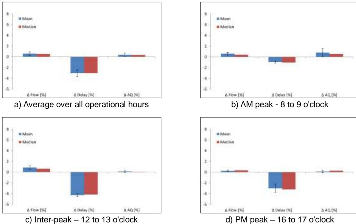
Figure 3 – System optimizing signal timings for two junctions in Leicester, UK, (a) over all operational hours (7 AM to 6 PM), (b) during AM peak hour (8 to 9 AM), (c) during the day (12 to 1 PM), (d) during PM peak hour (4 to 5 PM) during the demonstration period. Values are given in percent change from prediction.
