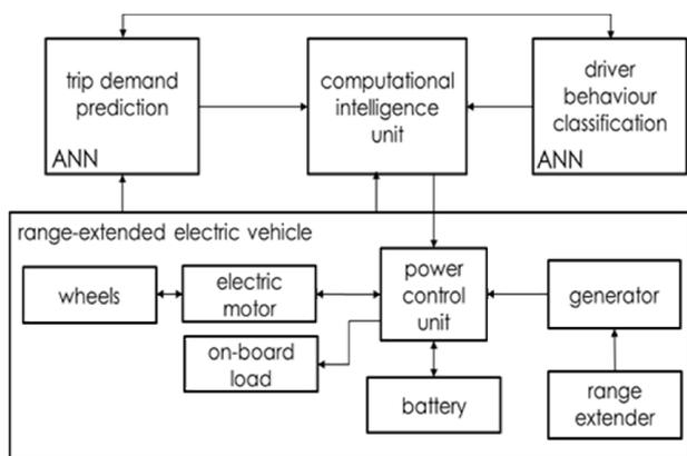
Fig. 7 Illustrating the proposed REEMS architecture.
