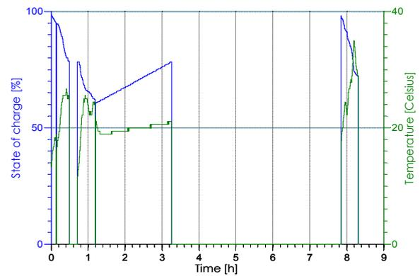
Fig. 5 Batteries temperature and state of charge acquired via OBD device.
