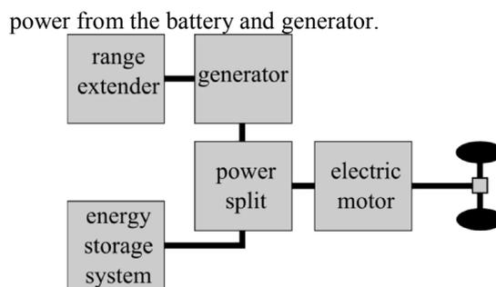
Fig.1 A schematic of powertrain configuration in a series hybrid electric vehicle.
