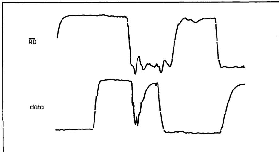
Fig. 5A Data output from 27C32 showing 1V switching spike on  $\overline{RD}$  line
