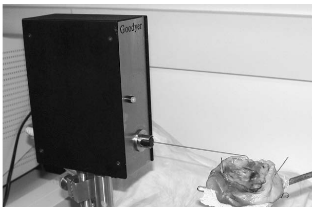
FIGURE 2. The LSR device as used for DSR measurements on hemilarynges.
